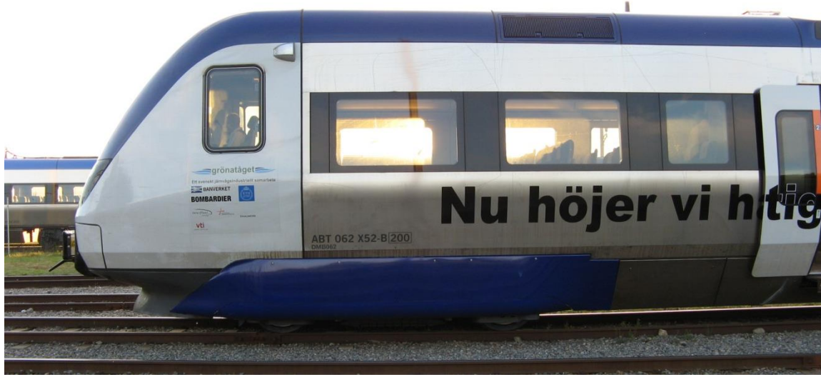
Figure 2: Gröna Tåget train, B-car with bogie skirts.
