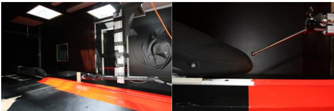
Figure 20: Pictures of the traversing system (left) and omniprobe (right). The omniprobe is placed in the (0,0) position in the right figure, such that the middle of the sphere is aligned to the tip of the tail.
